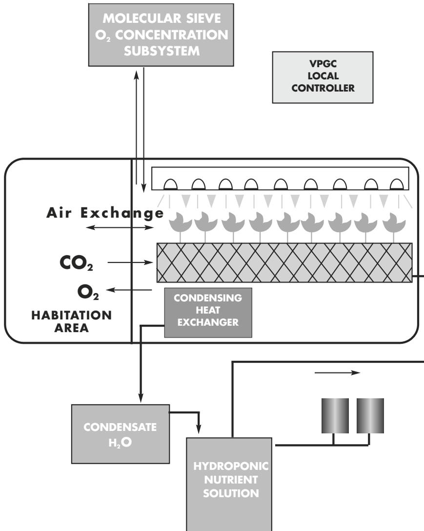
*Figure 2.1-2 The Phase I, 15-day test functional schematic*
