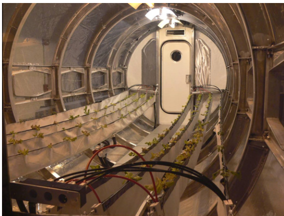
Fig. 2. Cable culture soilless hydroponic system deployed inside the LGH. Flexible plastic film envelopes were suspended from both ends of the LGH with a cable.
